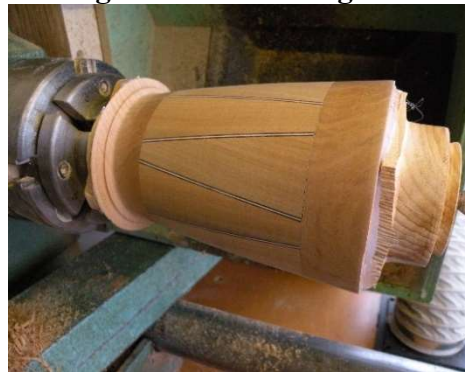
Mount on Base glue block, clean up outer profile using tailstock support to aid rigidity.
