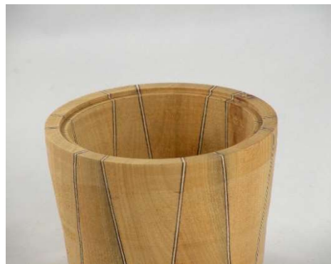
As end grain is involved, the use of tenon joints to strengthen the bond against wood movement is prudent.
