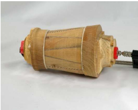
Glue up main components, the tenons aiding location and preventing mis-alignment. Glue blocks retained to facilitate final turning.
