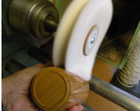
Apply wax, in this instance Microcrystalline.
