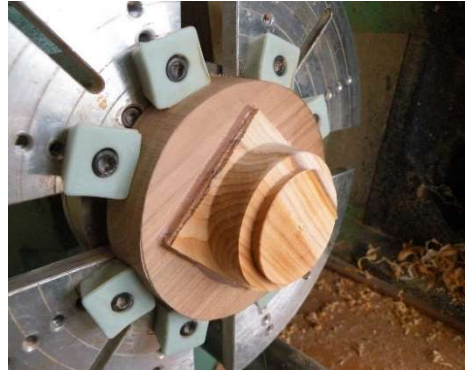
If necessary, due the thin section as in this case, mount them on Hot Melt Glue Blocks to aid holding whilst machining.
