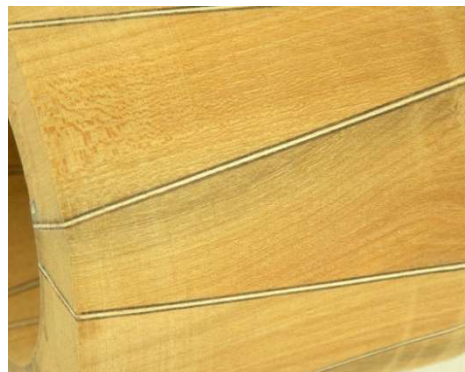
Check the glue joint line quality.
