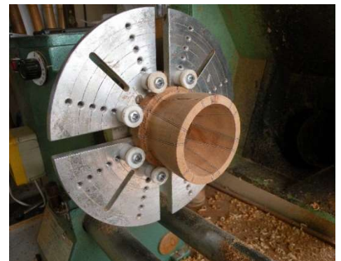
Next stage is to form basic body profile and prepare mating joint surfaces.
