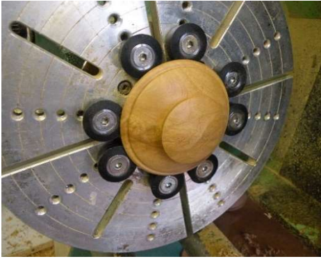
Reverse mount Lid and finish as far as sanding sealer.
