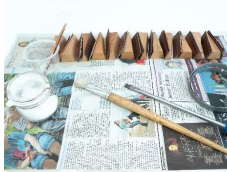
As Segment gluing can take 15-20 min., (48 pieces in this instance) a suitable working time adhesive is needed before firm clamping can be applied, essential if tight joints are to be achieved.
