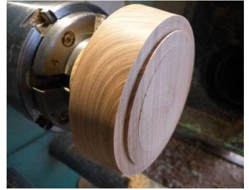
Turn matching tenons or sockets on Base and Top to locate with main body joints.
