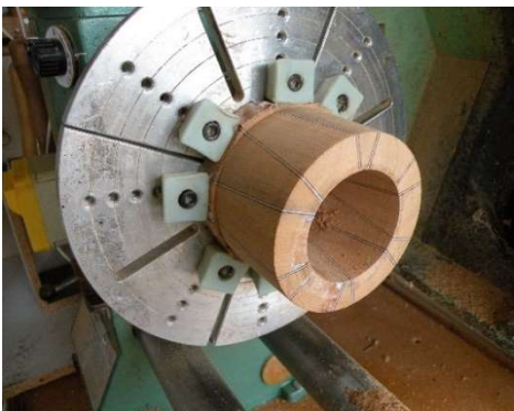
True up the basic body cylinder.
