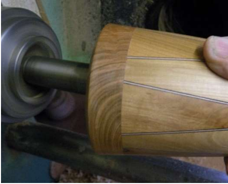
Abrade sealed body and lid with domed and large buffing mops
