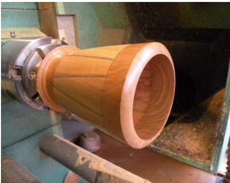
Finish internal and external turning to suit lid location, finish sanding as far as possible, and apply sanding sealer, part off from glue block.
