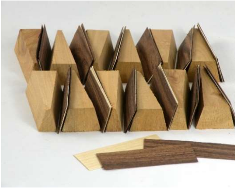
Cut sufficient joint highlight pieces, check segment grain character and adjust position sequence to balance final appearance.
