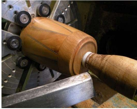
Reverse mount Main body, turn base detail.
