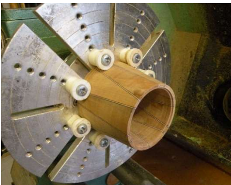
Always endeavour to sequence turning so that segmented forms are held in compression.
