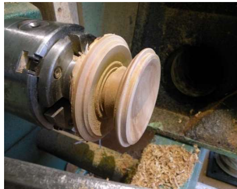
Mount and form lid profile to mate with the main body.
