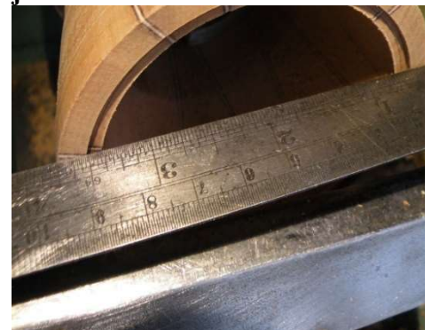
It is important that these joint faces are flat across the face if close fitting joins are to be achieved.
