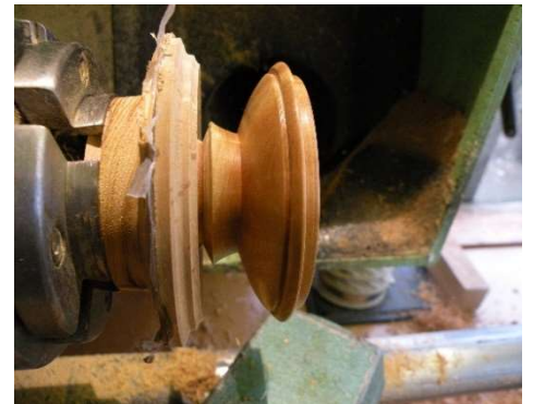
Sand and finish as far as possible with sanding sealer, part off.
