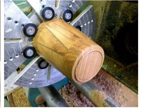
Sand and finish as far as sanding sealer.
