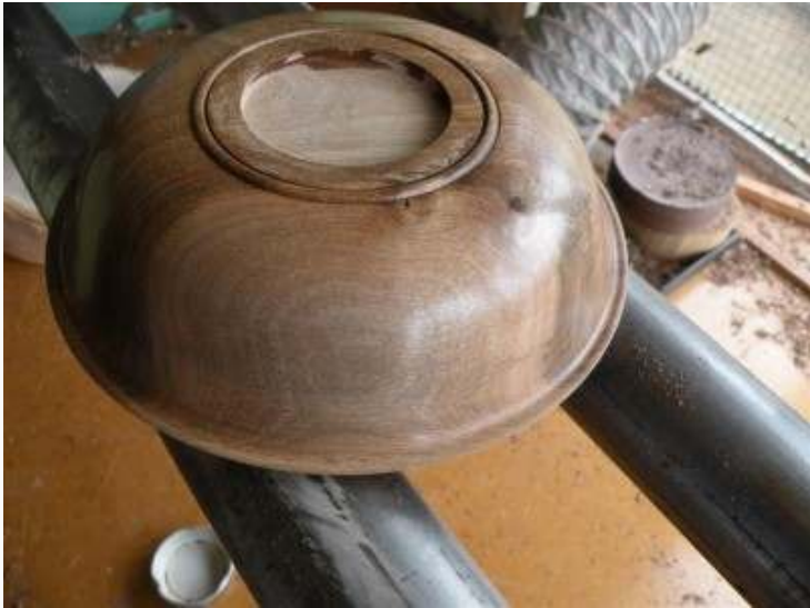
Sanding sealer brushed on and burnished with the cotton cloth used to wipe off surplus. Note: - This is the point where any sanding scratches will most likely make themselves known.
