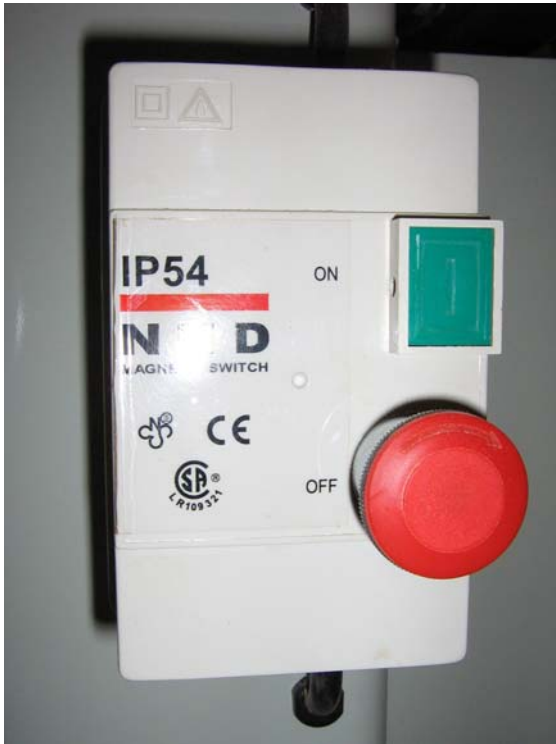
Figure 16 & 17 Single Phase DOL starter that is still based on a three pole switch inside.
