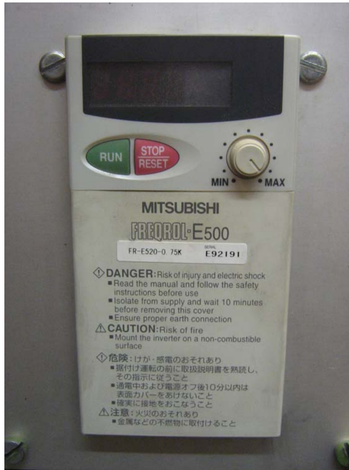
Figure 30 A Mitsubishi 1hp Inverter used on my bandsaw.
