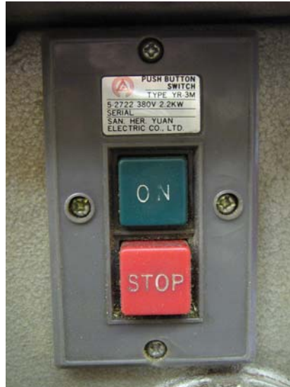
Figure 20 – A simple switch – Not NVR!
